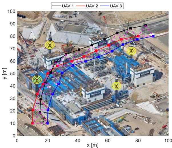
Figure 10. MAV paths on a construction site.
